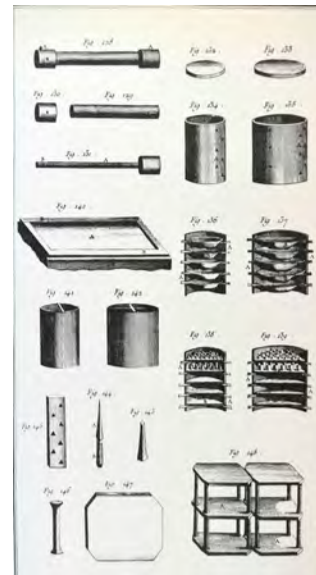
Fig. the types of saggars in "l'art du potier" Duhamel de Monceau (M)–Paris 1773
